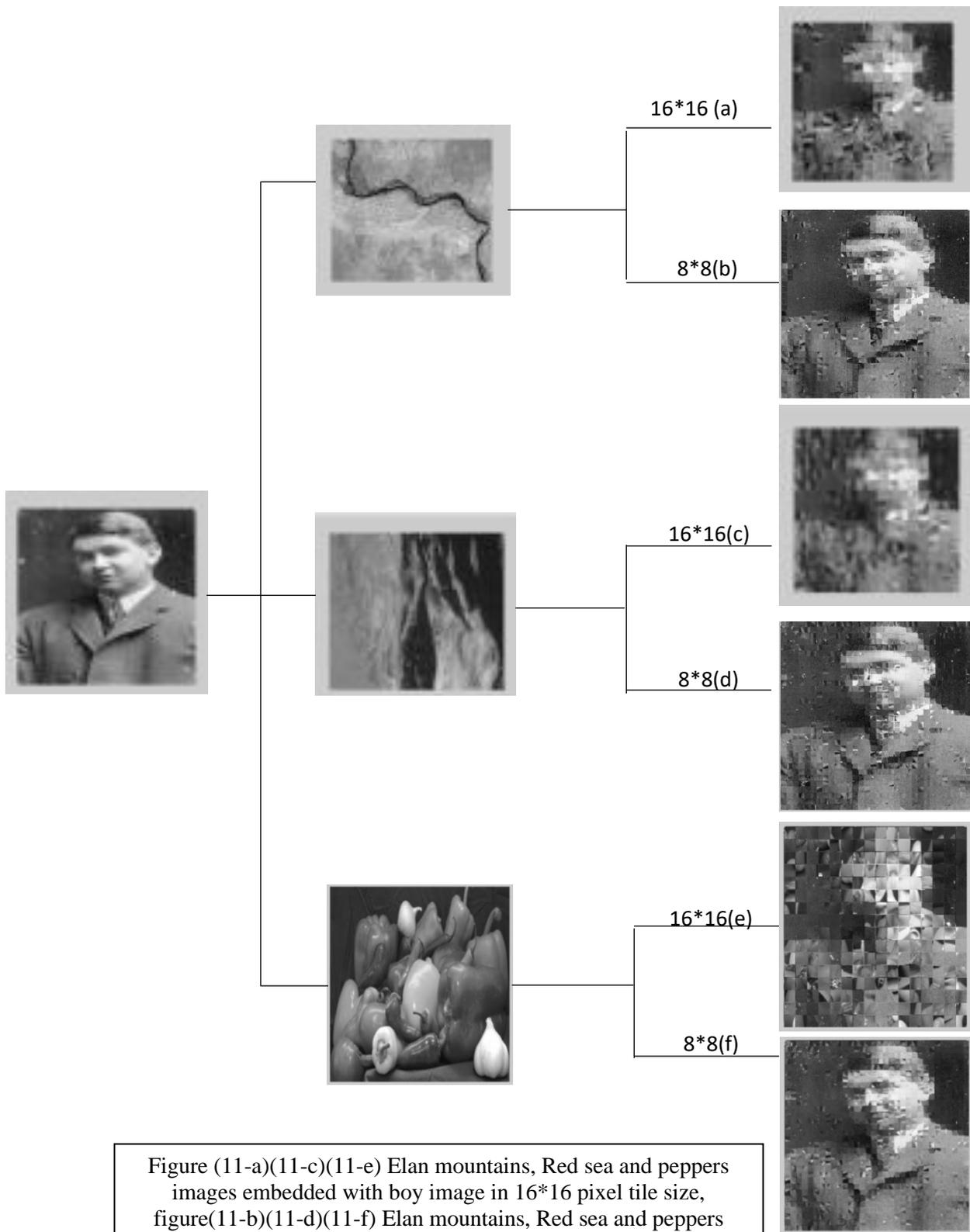
Observing the results, it is obvious that the image whose tiles are segmented by 8\*8 gives a higher resolution than the one which is segmented 16\*16. Mere observation is not enough to measure clarity and fussiness of each image and finding the optimal image in the embedding. Two measures have been used in this research, the first to measure the ratio of error in the image(MSE). The second measure is used to measure the noise (SNR) as follows:
