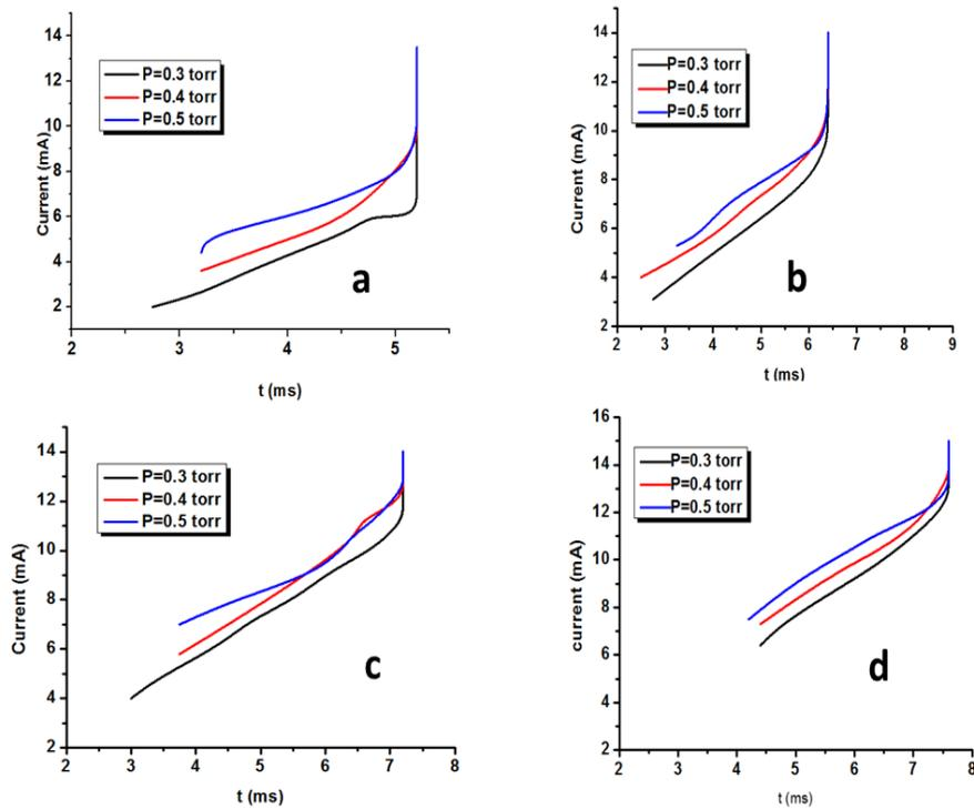
**Figure (4)** shows the discharge current against the decay time with inter electrodes distance  $1.5\text{ cm}$  at different pressure values.
