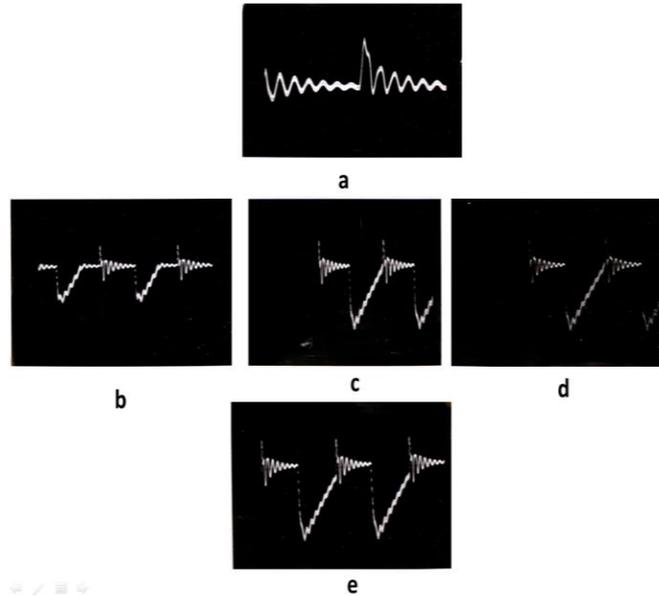
**Figure(5)** manifests (or you can say 'shows') the voltage and current pulses photographs, (a) spike voltage pulse shape b, c, d and e represent the pulse current pictures and give the stages of the time growth of pulse glow discharge current at pressure 0.3 torr the inter electrodes distance is 1.5 cm and  $T_W = 5.2 \text{ ms}$ .
