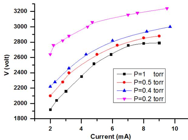
**Figure (6)** shows I-V characteristics for argon discharge in different pressure values at  $d=1.5 \text{ cm}$  and  $T_W = 5.8 \text{ ms}$ .
