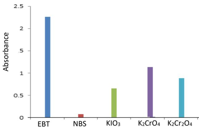
Figure 3: Effect of 1 mL of  $5 \times 10^{-3} \text{M}$  oxidant on the bleaching of  $100 \mu\text{g mL}^{-1}$  EBT
