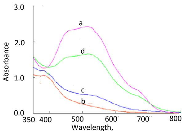
Figure 1: Absorption spectra of  $100 \mu\text{g mL}^{-1}$  EBT in the presence of a base (a) in the absence and (b) in the presence of  $5 \times 10^{-3} \text{M}$  NBS with (c)  $2 \mu\text{g mL}^{-1}$  and (d)  $6 \mu\text{g mL}^{-1}$  of Paracetamol.
