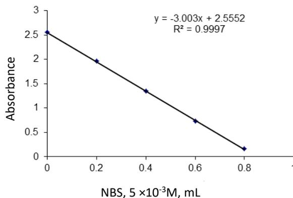
Figure 4: Effect of NBS concentration on the decolorization of  $100 \mu\text{g mL}^{-1}$  EBT
