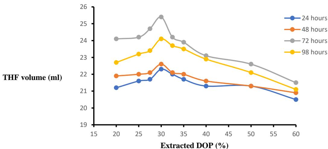
**Figure 1. THF volume and extracted DOP at different temperatures for PVC plastic products before manufacturing.**
